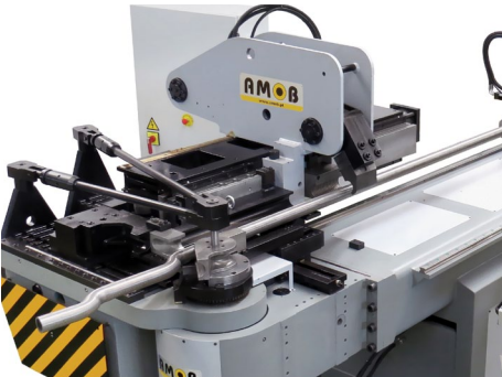
Booster bending The pressure die assist/booster cylinder is integrated into the pressure die carrier head.
