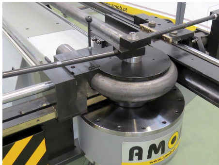
Direct acting pressure die cylinder Pressure die cylinder is mounted in tube's centerline plane to resist the bending forces.
