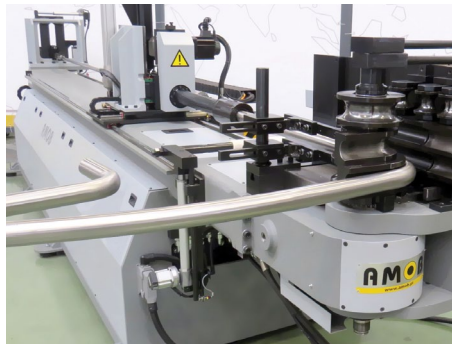
Fixed and variable radius All Ce CNC R models have multi-stack, fix and variable radius capability.
