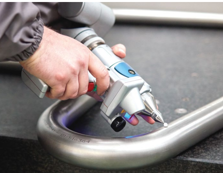
3D imaging devices connection Allows easy CAD comparison, dimensional analysis and reverse engineering.
