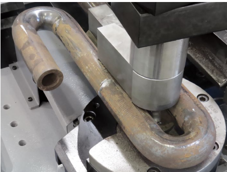
Serpentine tooling Designed to exact centerline radii specifications requiring continuous 180-degree plane change.
