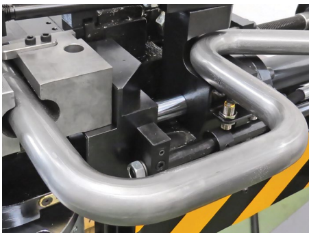
Special propose tooling On request, MDH series may be equipped with special tooling.
